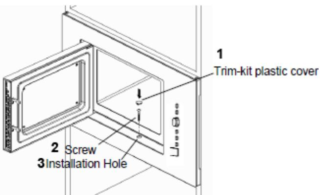
Open the door; fix the oven to the cabinet with screw at the installation hole. Then fix the trim-kit plastic cover (1) on the screw (2) in the installation hole (3).
