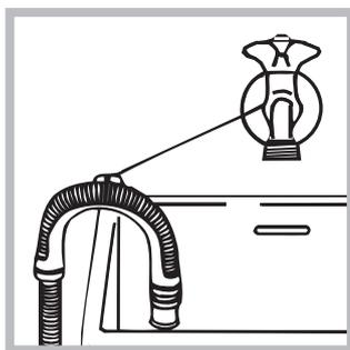
alternatively, placed it over the edge of a basin, sink or tub, fastening the duct supplied to the tap (see *figure*). The free end of the hose should not be underwater.
