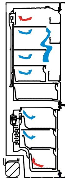
In fridges with new-generation cooling technology, a fan blows dry cold air evenly throughout the fridge and freezer compartments. The cold air cools your food evenly and uniformly, preventing humidity and ice build-up.
