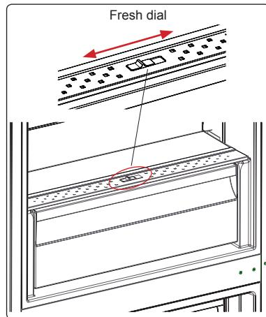
If the crisper is full, the fresh dial located in front of the crisper should be opened. This allows the air in the crisper and the humidity rate to be controlled, to increase the life of food within.
