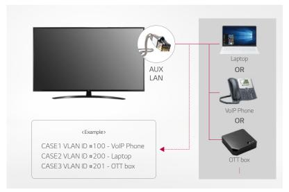
\* AUX LAN (LAN out) ID: Set a VLAN ID to be assigned to external devices connected to the LAN out port. (An AUX LAN is used for assigning a VLAN ID.)
