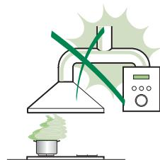
Connect the extractor to the exhaust flue through a pipe of minimum diameter 120 mm. The route of the flue must be as short as possible.
