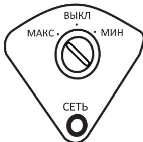
The temperature is regulated by turning the thermostat to the appropriate position (from MIN to MAX).
