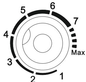
**ATTENTION!** It is not recommended to use the chest freezer for more than 24 hours in quick freeze mode. It is recommended that after 24 hours, turn the thermostat control to any position below the maximum.
