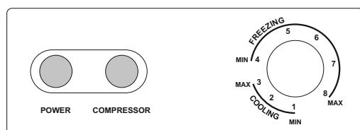
A green light on the control panel indicates that the compressor is on and running.
