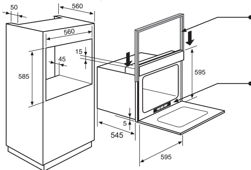
● Protection trim (supplied with the oven when necessary)
