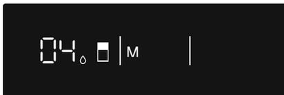
Press cooler set button (#4 on control panel diagram) until Super cool symbol (#3) will be seen on the screen. Buzzer will sound beep beep. Mode will be set.
